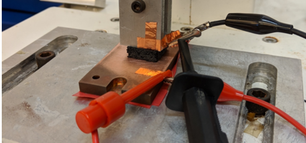
Figure 4-2 Sandwich structure for testing tactile sensors. Copper tabs allow alligator clips a better place to grip. Copper plate required sanding between tests to maintain a clean surface.
