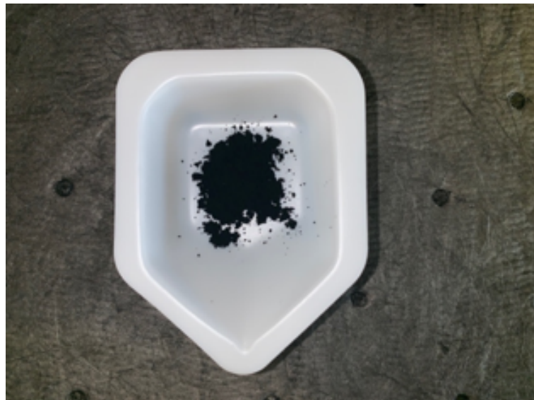
Figure 1-7 MW-CNTs in weigh boat, 95% purity, 10-20 nm dia. 10-30 \mu\text{m} length.
