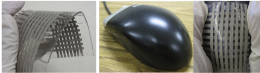
Figure 1-2 Silver/PDMS flexible skin-like sensors (top) response as pressure is applied, (bottom) being flexed around a computer mouse [15].
