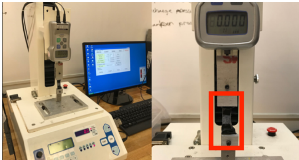
Figure 3-3 SHIMPO tabletop MTS set up. Sample under no load, prior to testing, is placed into testing set up. Duct tape wrapped around the ends provides a gripping point for the clamps that does not deform the sample.
