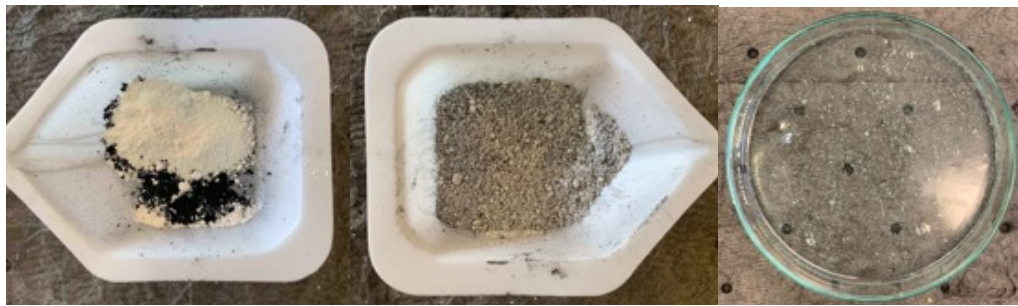
Figure 2-1 ZnO and CNT nanopowders before (left) and after mixing (middle); PDMS before de-bubbling (right).
