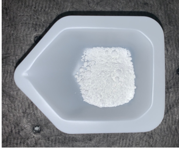
Figure 1-8 ZnO, 29 nm, 99.5% purity in weigh boat.
